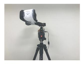
Figure 8: Our VR testbed consists of a GearVR, an S7, a Pan/Tilt mount, a 3D-printed holder for the mount, a Raspberry Pi to accurately control the mount's motion, and a tripod for stabilizing the test instruments.
